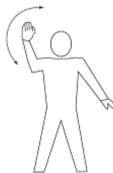
Point left arm downward, right arm repeatedly moved upward-backward. Speed of arm movement indicating rate of turn. TURN TO THE RIGHT
